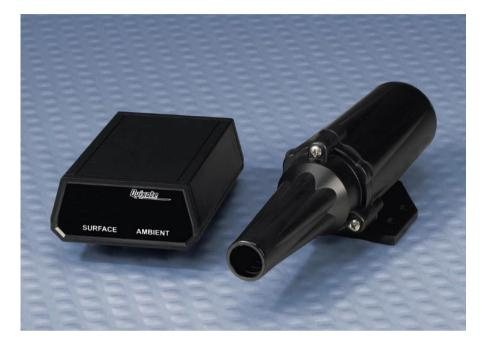
The Vaisala Surface Patrol Pavement Temperature Sensor with Display DSP100 Series is a mobile temperature sensor used to detect possible freezing temperatures on the pavement. It features a noncontact infrared sensor for measuring pavement temperature, and also measures air temperature. The easyto-use DSP100 is valuable for large agencies, such as Departments of Transportation, all the way down to smaller companies with only a few trucks.
