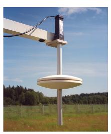
PTB210 paired with SPH10 static pressure head
