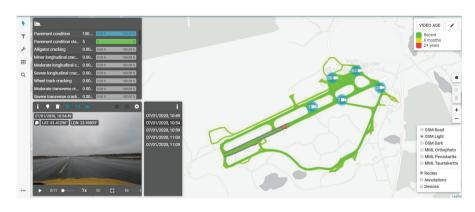
RoadAI makes it easy to collect, view, and leverage runway condition data on a map.
